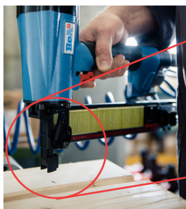
Safety Yoke Deactivated Shooting not possible
